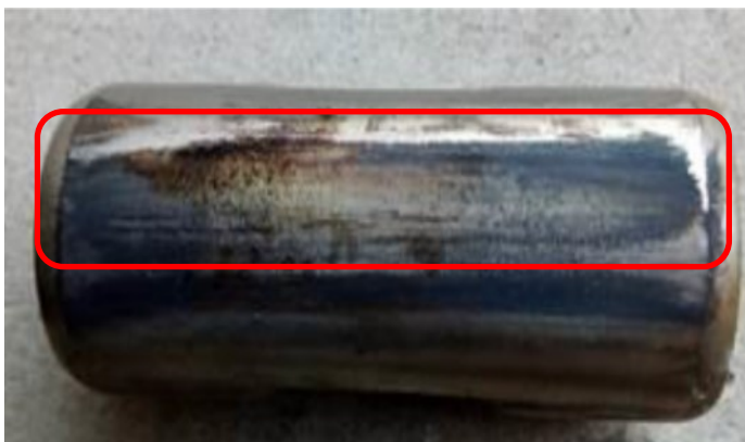
Spray metal coupling and Boronized tubing wear
