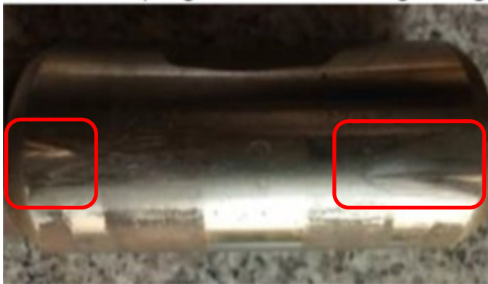
Spray metal coupling and Composite Plated Tubing (Q2-CPT) wear
