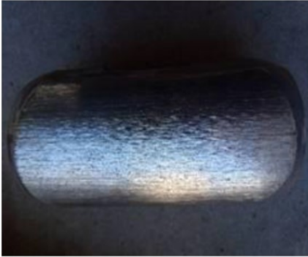
T-type coupling wear from testing against L-80 tubing
