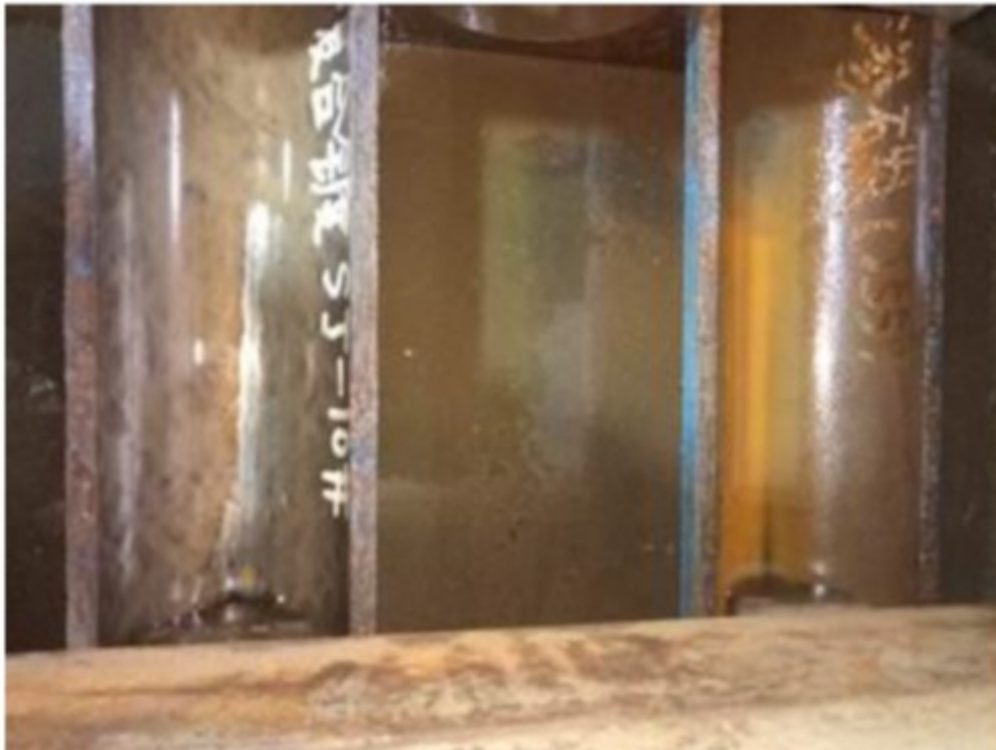
T-type coupling wear from testing against L-80 tubing
